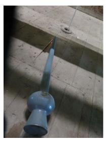
On 16th July the tenor clapper broke whilst the bells were being rung down after service ringing. There was a tremendous thump as the clapper hit the bell chamber floor. Investigation the following day showed that the clapper had broken a few inches from the pivot (see picture top right) where, judging from the discolouration, there had been a long standing crack in the shaft. On landing the clapper had broken a ringing chamber floor board (see picture on bottom right).
